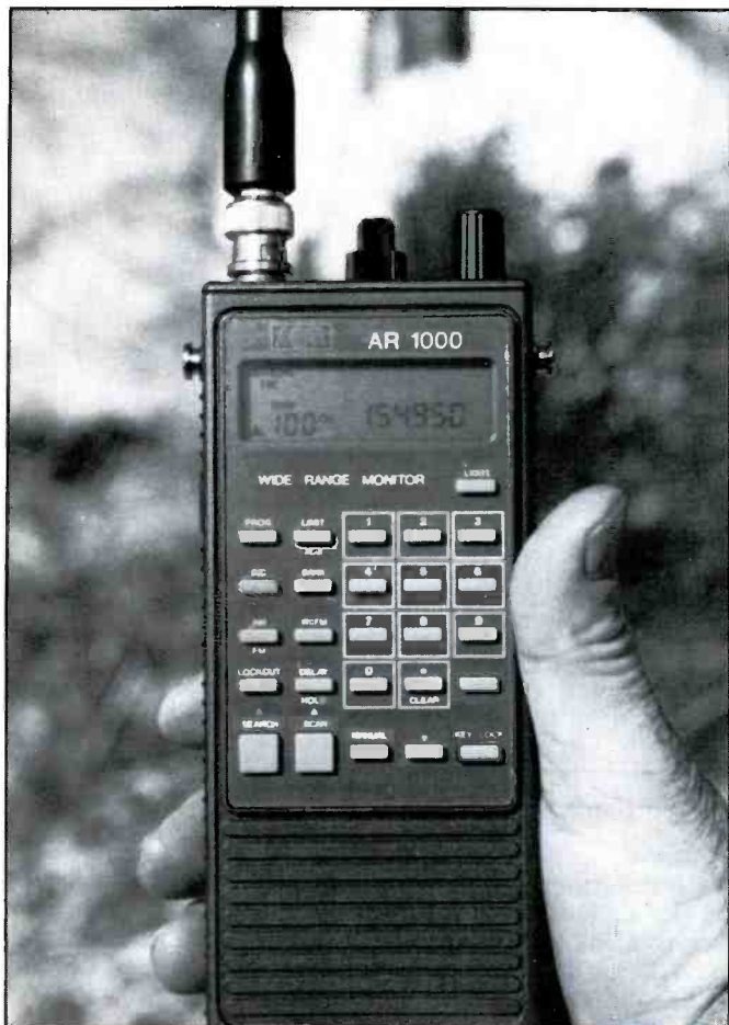
A handheld is helpful for tornado monitoring since it has a self-contained power supply and a built-in battery.
