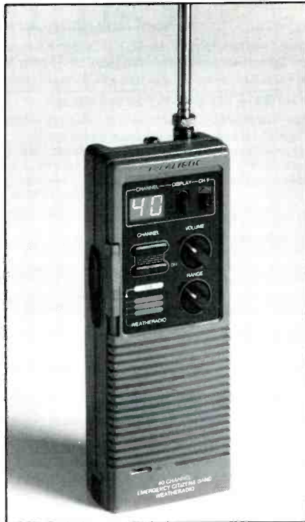
The Realistic TRC-475 is a convenient emergency CB rig that also receives three NOAA weather frequencies.
