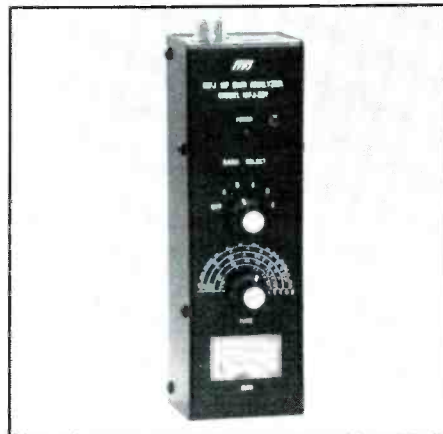
This MFJ SWR analyzer is actually a micro-watt HF or VHF transmitter with an auto-calibrating SWR bridge built-in.
