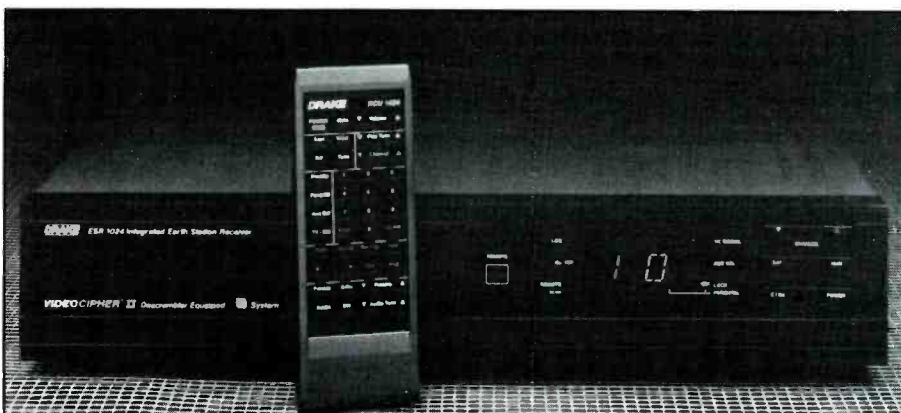
The ESR 1024 from RL Drake is an integrated Earth Station Receiver with a VideoCipher II descrambler equipped system.
